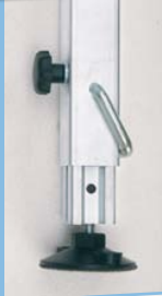
Telescopic platform legs with grid, adjustable with safety stirrups, additional height adjustment, c. 40 mm, through polyamide load balancers
