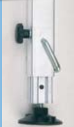
Telescopic platform legs with grid, adjustable with safety stirrups, additional height adjustment, c. 40 mm, through polyamide load balancers
